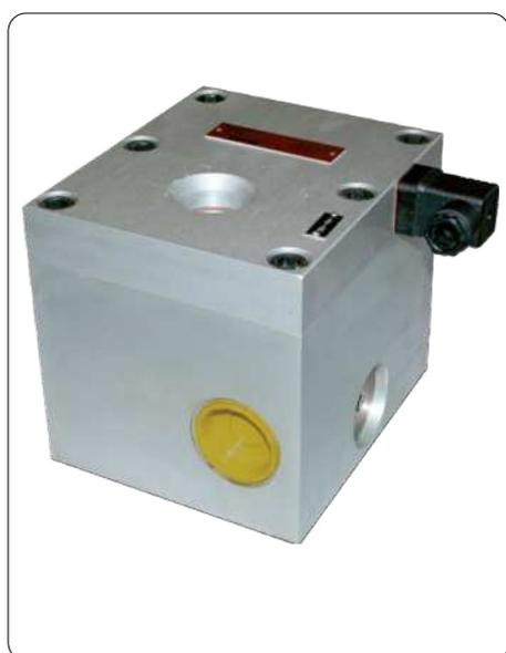
Flow limiters are used in circulating-oil lubrication systems. The task of a flow limiter is to divide up the volumetric flow of the main line into parallel individual volumetric flow quantities and to “limit” these according to requirements, or to keep them constant. The volumetric flow produced does not depend on the system pressure and is nearly independent of viscosity.
