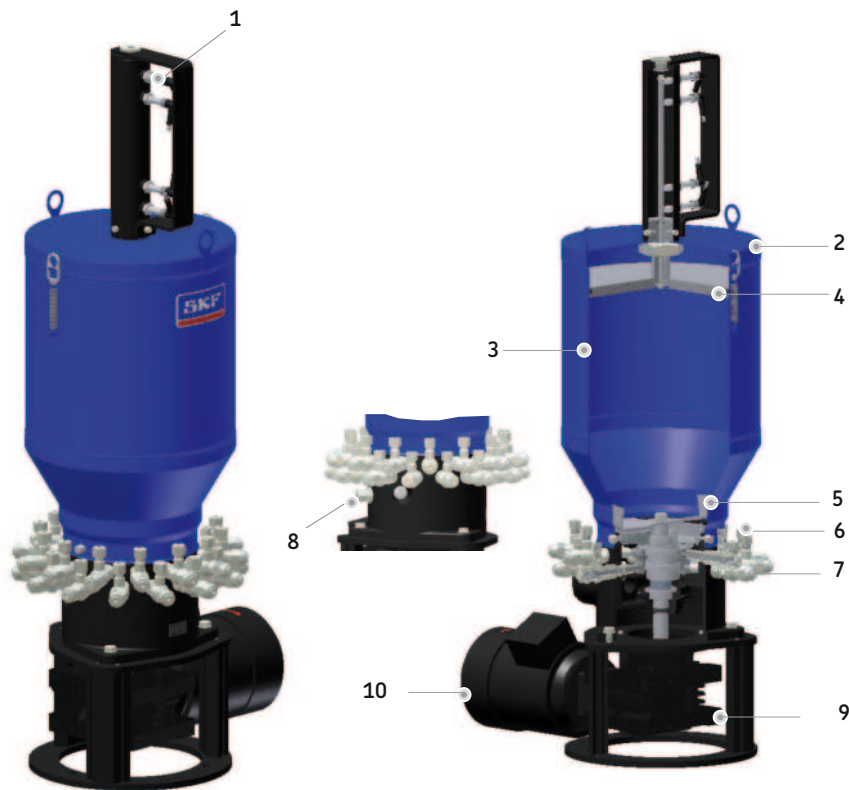
Components of the FB, FB-ATEX unit, Fig. 1
