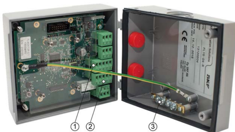
Figure 26 Connectors for CAN bus in monitor, 1: X12, 2: X13, 3: TE-Bar
