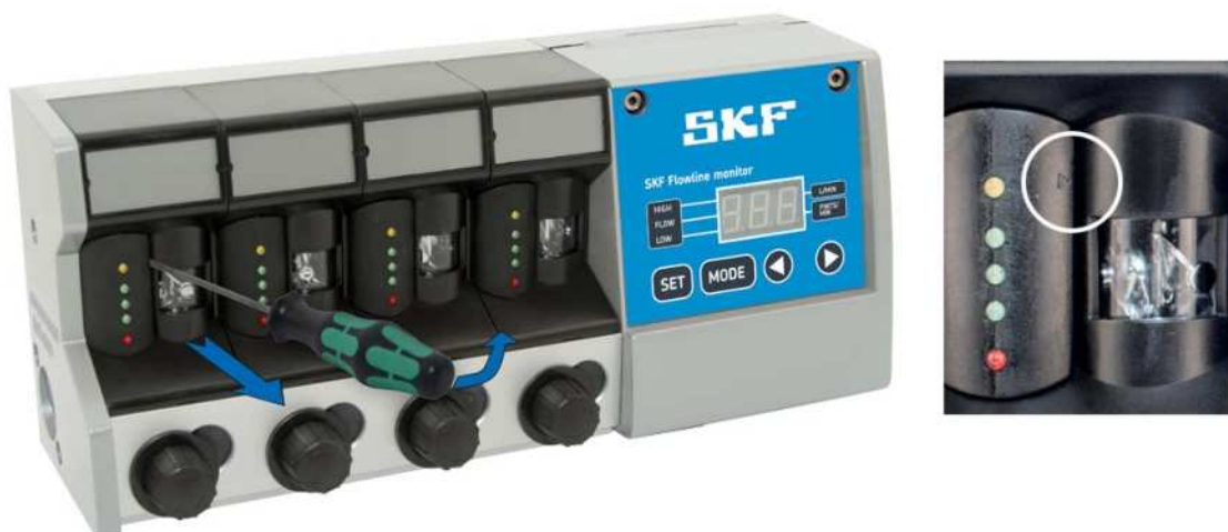
Figure 18 Removing sensor. Spare part: Sensor unit ( Refer to section 16 Spare parts ).
