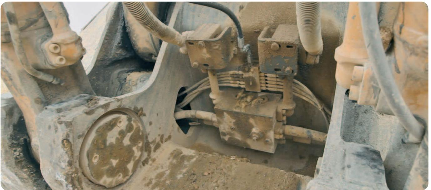
The electrical HCC hose connection control is a monitoring and signalling unit to reliably check lubricant feed lines for breaks. This unit shows the driver or operator of the machine immediately if there is a fault by sending a collective fault signal.
