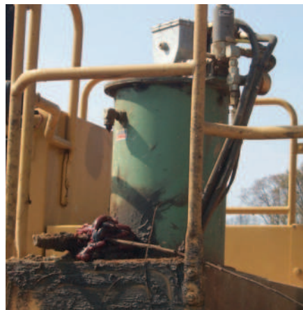
Example of reservoir overfilling that can cause slip-and-falls, fire hazards or other concerns.
