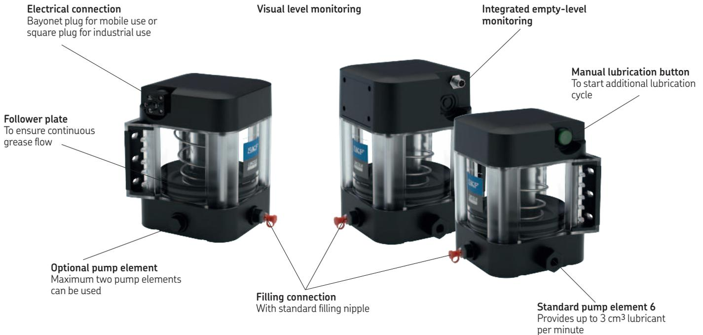
The Lincoln Compact progressive pump (CLP) series has different monitoring options. CLP Basic Plus variants feature integrated empty-level monitoring that informs the user before the pump runs out of lubricant.
