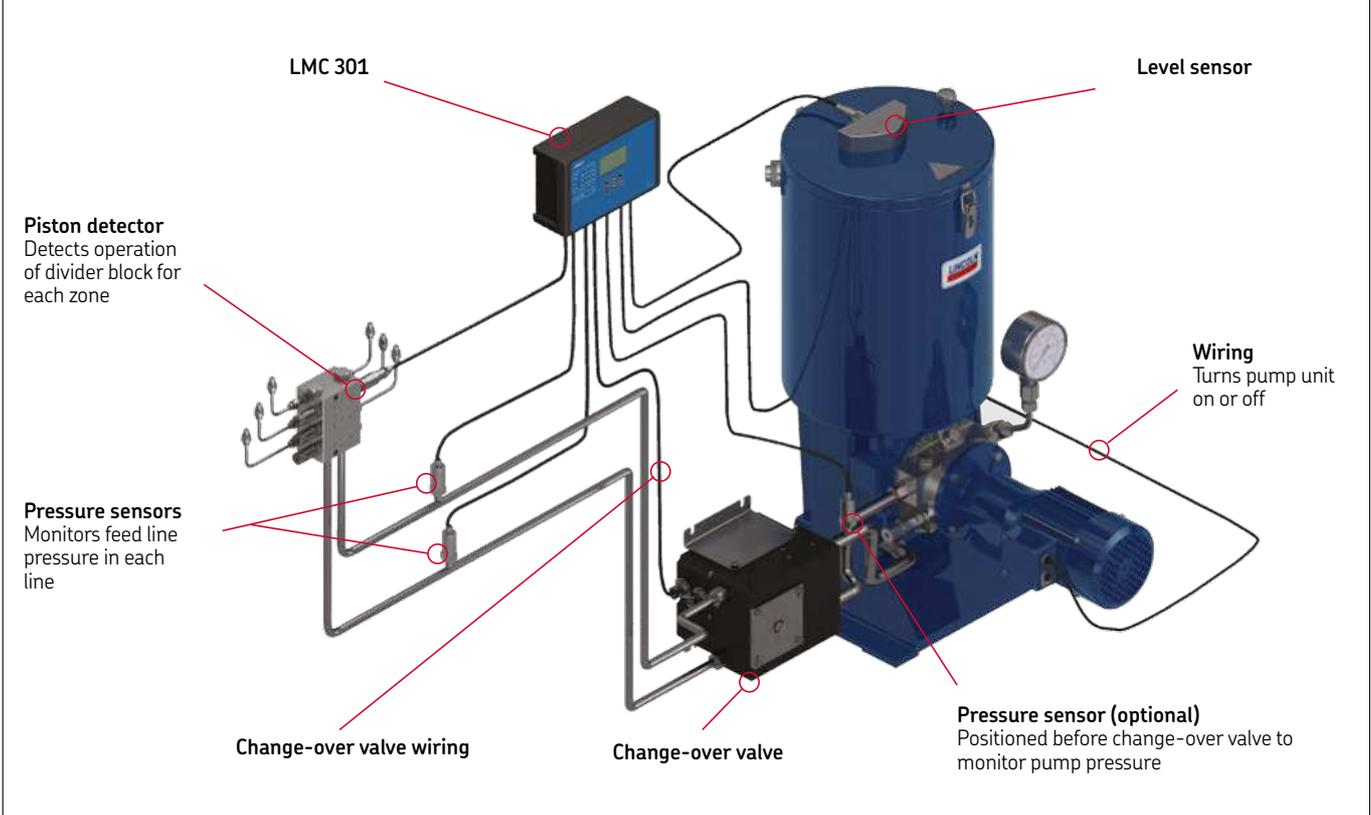
Dual-line lubrication systems, including SKF DuoFlex and Lincoln Helios, utilize two main lines that are supplied alternately with lubricant from a high-pressure pump via a change-over valve, whereby the lubricant also serves as a means of control for the system. These systems are suitable for applications with many lubrication points over long distances in harsh environmental conditions.
