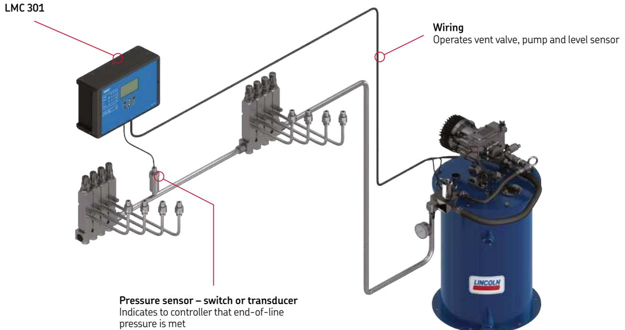
Regardless of the application, the principle of single-line lubrication remains the same: a central pump station automatically delivers lubricant through a single supply line to the lubricant metering device. Each metering device serves only one lubrication point and may be adjusted to deliver the precise amount of grease or oil required. Systems can service one machine, different zones on one machine or even several separate machines.
