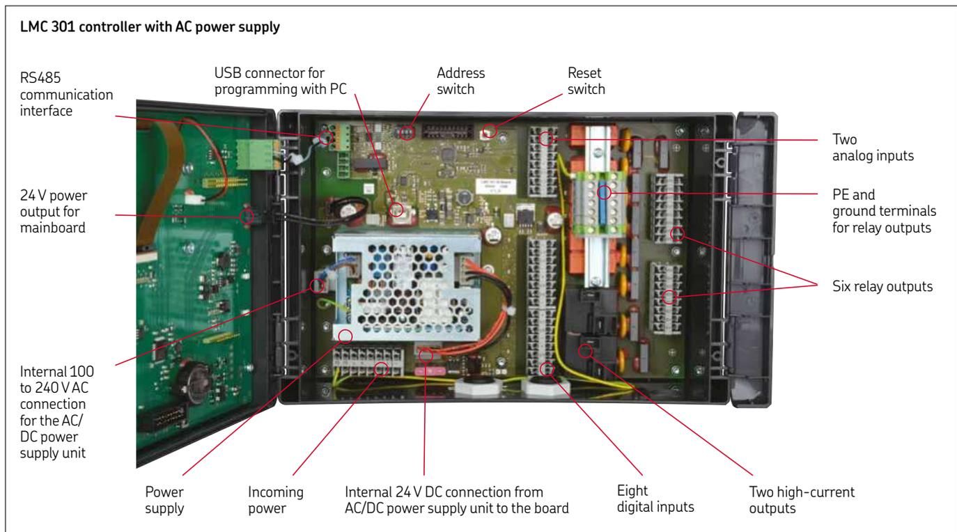
Designed for use with pumps that have no internal controller, the LMC 301 is suitable for applications where sophisticated control and feedback are required. This versatile controller can handle multiple configurations and diverse temperature ranges.
