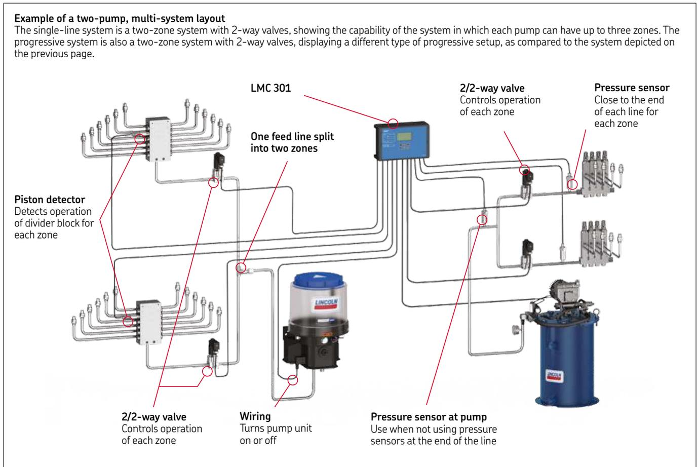
The LMC 301 controller allows for use of up to three pumps, and each pump can operate up to three zones. Each of the pumps can be used with a different system type. Therefore, one unit could operate a single-line system pump and a progressive system pump or a progressive system pump and a dual-line pump.
