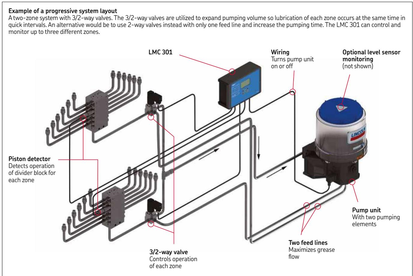
In progressive automatic lubrication systems, a piston pump supplies a defined amount of lubricant through the main line to the metering device that serves each outlet. SKF ProFlex and Lincoln Quickclub systems are designed for specific applications and can be configured to meet the unique requirements of every lubrication point on the equipment.
