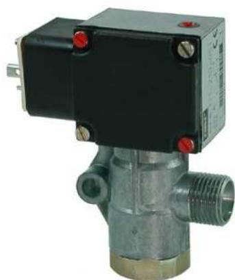
Flow monitors/sensors have the task of monitoring the flow of lubricant from the pump or a piston distributor element to the lube point. Flow monitors with various designs are used for this job. A further task involves monitoring a continuous flow of oil from a pump through a lubrication system. These flow monitors are designed for a throughput ranging from 0,5 cm<sup>3</sup> to 14 000 cm<sup>3</sup>.
