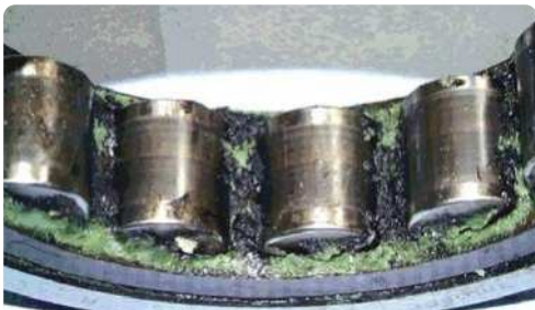
Lubricant degradation caused by electrical discharge currents
