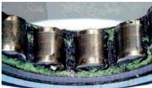
Lubricant degradation caused by electrical discharge currents
