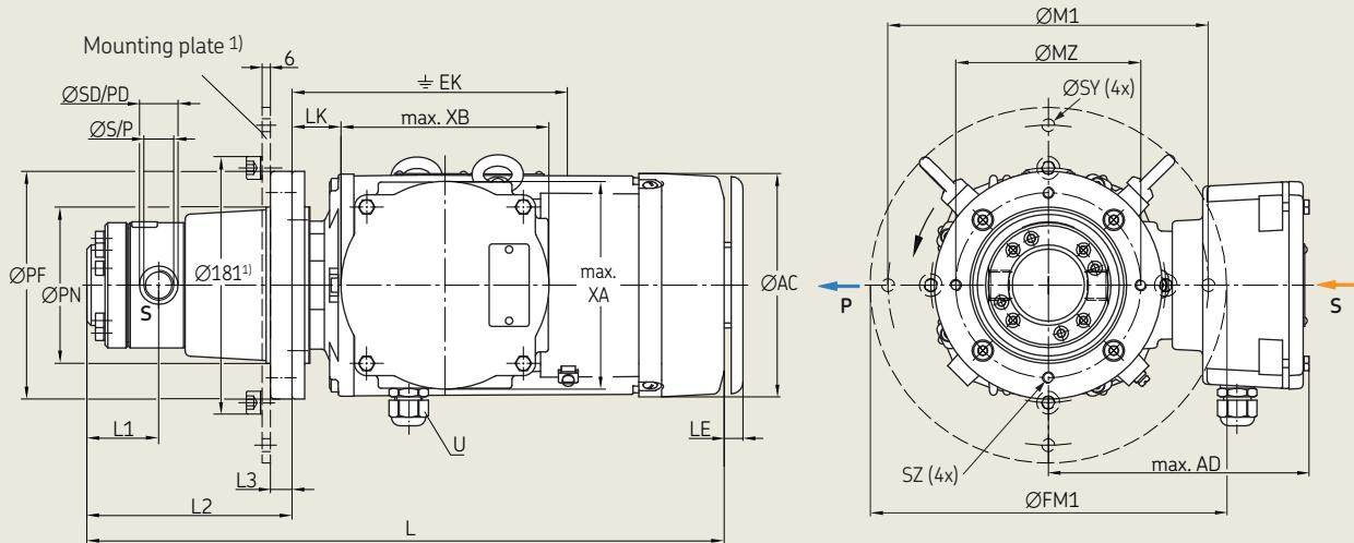
1) Mounting plate only for delivery rate 30, 40, and 50 l/min.
