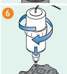
If the support flange is not mounted on the application, screw the complete lubricator onto the application. Your lubricator is ready.
