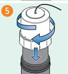
Screw the drive unit cap onto the cannister.
