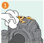
Clean the lubrication point from dirt and old grease in such a way that the dirt is not entering the lubrication point itself.
