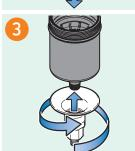
Screw the support flange on the cartridge until is it is fixed.
