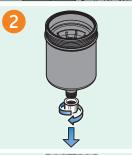
Remove the yellow protection cap from the new grease cannister.
